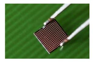
The chip is composed of three or more processors that are stacked vertically and connected together -- resulting in increased speed and multitasking, more memory and calculating power, better functionality and wireless connectivity. Credit: EPFL / Alain Herzog
