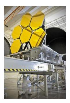
The first six flight-ready James Webb Space Telescope's primary mirror segments are prepped to begin final cryogenic testing at NASA's Marshall Space Flight Center in Huntsville, Ala. Credit: NASA/Chris Gunn
