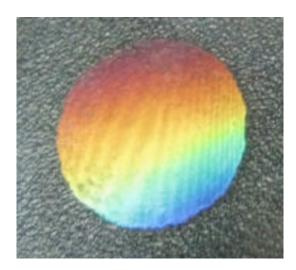
Biomimetic graphene oxide with iridescence like a butterfly's wing and superhydrophobicity like a rose petal. Image credit: Wang, et al. ©2012 Chemistry - An Asian Journal
