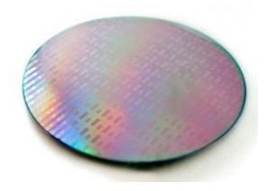
Silicon wafer with photonics biosensorchips.
