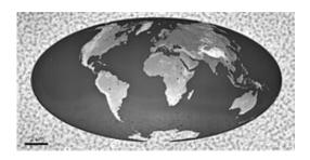
The map, produced on a tiny sliver of polymer, measures just 22 by 11 micrometers. To put that into perspective, 1000 copies of the map could fit within a single grain of salt.
