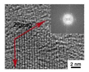
This transmission electron microscope image shows a graphene quantum dot with zigzag edges. The quantum dots can be created in bulk from carbon fiber through a chemical process discovered at Rice University. (Credit: Ajayan Lab/Rice University)
