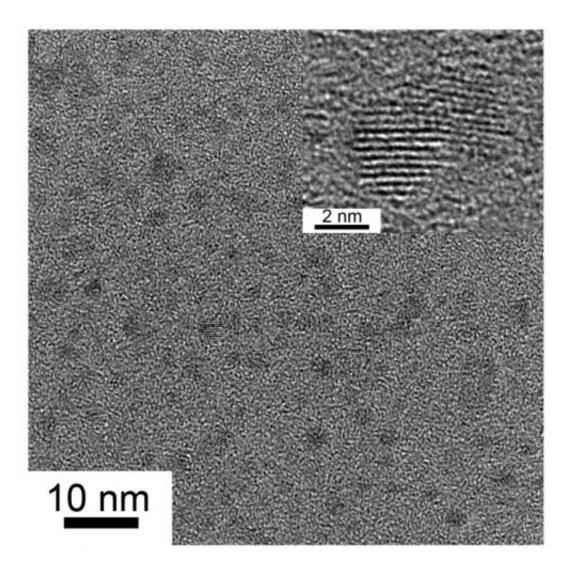
Dark spots on a transmission electron microscope grid are graphene quantum dots made through a wet chemical process at Rice University. The inset is a closeup of one dot. Graphene quantum dots may find use in electronic, optical and biomedical applications. (Credit: Ajayan Lab/Rice University)
