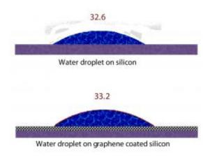
Drops of water on a piece of silicon and on silicon covered by a layer of graphene show a minimal change in the contact angle between the water and the base material. Researchers at Rice University and Rensselaer Polytechnic Institute determined that when applied to most metals and silicon, a single layer of graphene is transparent to water. (Credit: Rahul Rao/Rensselaer Polytechnic Institute)
