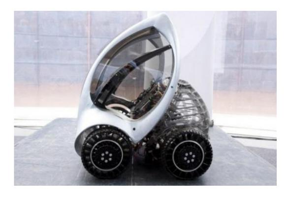
The "Hiriko", the Basque word for "urban", is an electric two-seater whose motor is located in the wheels and which folds up like a child's collapsible buggy, or stroller, for easy parking.
