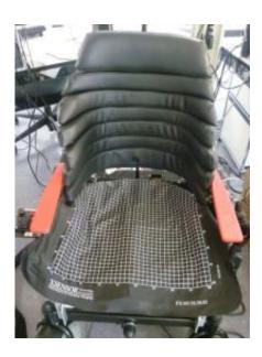
The pressure mat on the wheelchair seat measures how the backrest "forces" users to change their sitting position, thereby shifting the location of pressure points.
