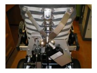
The backrest of the seat shell (seen from behind) is constructed of ribs and joints which simulate the structure of a human torso.
