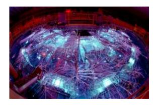
The Z Machine at Sandia National Labs generates bursts of x-rays that scientists have used to replicate the temperature and density conditions in white dwarf stars. Credit: Z Machine Collaboration, Sandia National Lab, Lockheed Martin, NNSA, DOE
