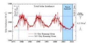
A graph of the sun's total solar irradiance shows that in recent years irradiance dipped to the lowest levels recorded during the satellite era. The resulting reduction in the amount of solar energy available to affect Earth's climate was about .25 watts per square meter, less than half of Earth's total energy imbalance. Credit: NASA/James Hansen
