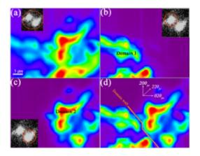
Diffraction intensity contrast maps for Fe0.94O measured at 24.7 GPa. From Yang Ding et al., Appl. Phys.Lett. 100, 041903 (2012).
