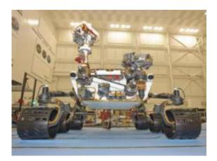
The Curiosity rover, which lifted off Nov. 26, 2011, will arrive at the Red Planet in August 2012. The rover, shown here during testing inside the Spacecraft Assembly Facility at the Jet Propulsion Laboratory in California, is about the size of a Mini Cooper and weighs roughly five times as much as the Spirit and Opportunity rovers. Credit: NASA/JPL-Caltech
