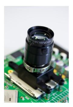
Imec's prototype camera with imec's hyperspectral sensor.
