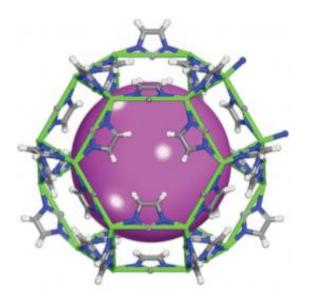
This illustration of a metal-organic framework, or MOF, shows the metal center bound to organic molecules. Each MOF has a specific framework determined by the choice of metal and organic. Sandia chemists identified a MOF whose pore size and high surface area can separate and trap radioactive iodine molecules from a stream of spent nuclear fuel. (Image courtesy of Sandia National Laboratories)
