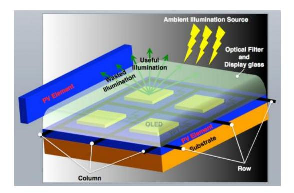
A thin-film system harvests energy from wasted light in an OLED display. Image credit: Arokia Nathan (via IEEE)
