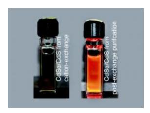
This shows the luminescence of CdSe/CuS nanocrystals prepared by cation-exchange. On the left are crystals prior to purification, on the right are the same nanocrystals after impurities have been removed. Credit: Courtesy of Berkeley Lab
