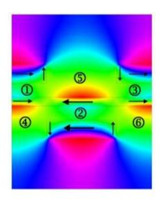
This is an illustration of Durdu Guney's theoretical negative-index metamaterial, which would be the heart of a perfect lens. The colors show magnetic fields generated by plasmons. The black arrows show the direction of electrical current in metallic layers, and the numbers indicate current loops that contribute to negative refraction. Credit: Durdu Guney
