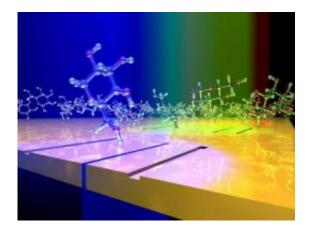
Each plasmonic interferometer -- thousands of them per square millimeter -consists of a slit flanked by two grooves etched in a silver metal film. The schematic shows glucose molecules "dancing" on the sensor surface illuminated by light with different colors. Changes in light intensity transmitted through the slit of each plasmonic interferometer yield information about the concentration of glucose molecules in solution. Credit: Domenico Pacifici, Brown University
