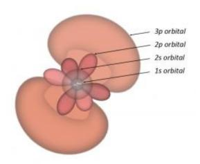
A neon atom has two electrons in the 1s orbital, two in the 2s orbital, and six in the 2p orbital; the 3 shell is normally unoccupied. In the first test of nonlinear multidimensional spectroscopy with neon, Belkacem's team will boost an electron in the relatively low-energy 2s orbital into the 3p orbital, an excited valence state. Within quadrillionths of a second a 2p electron will fill the 2s "hole," so that when the 3p electron relaxes, it will emit a photon signaling the transaction.
