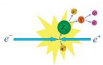
Figure 2. Production of Z_b in an electron-positron collision. Immediately after being produced, the Z_b decays into a bottomonium ( \Upsilon or h_b ) and a charged pi meson ( \pi^\pm ). The bottomonium then decays into a pair of muons ( \mu^\pm ), which are subsequently measured with a detector.
