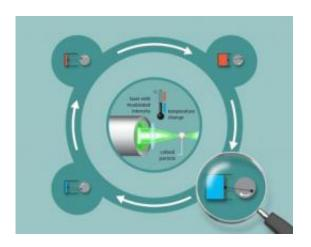
A Stirling engine in the microworld: In a normal-sized engine, a gas expands and contracts at different temperature and thus moves a piston in a cylinder. Physicists in Stuttgart have created this work cycle with a tiny plastic bead that they trapped in the focus of a laser field. Credit: Fritz Höffeler / Art For Science
