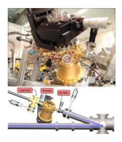
This chamber and attached apparatus (see diagram, bottom) are used to introduce various gases to test contamination build-up on multi-layer surfaces.
