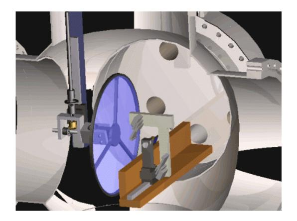
This animation shows how the researchers measure contamination that results when EUV photons (green and purple lines) strike a photoresist on a rotating wafer (purple disk), leaving deposits on the witness plate (gray diagonal structure in center of frame). Credit: Steven Grantham/NIST
