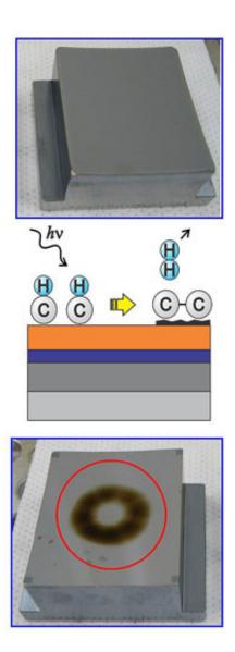
Contamination forms on a clean multi-layer surface (top) when EUV photons react (middle) with gases, resulting in carbonaceous deposits (bottom). Photos: SEMATECH
