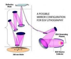
EUV lithography requires multiple mirrors (multi-layer Bragg reflectors) to position and focus the EUV beam.
