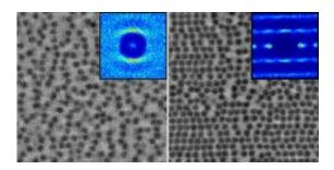
The black-and-white confocal microscopic images above show microscopic particles suspended in a viscous fluid, forming string-like structures while undergoing shear flow. The particles are less densely packed in the image at left. The inset color images visually represent the probability of finding a particle at a particular location if there is already a particle at center. Courtesy of Cornell University, Xiang Cheng
