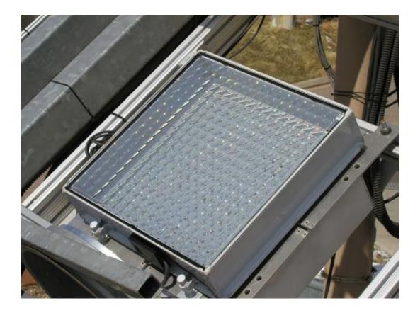
This solar cell module made by Semprius is being tested at NREL's Outdoor Test Facility. Credit: NREL staff
