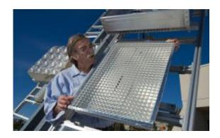
NREL scientist Keith Emery examines a Semprius solar module at the laboratory's Outdoor Test Facility. NREL helped Semprius characterize and test its tiny solar cells, which are the diameter of a dot made by a ballpoint pen. Credit: Dennis Schroeder
