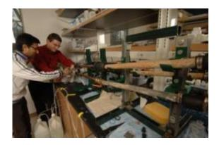
Old lead water pipes are spliced to brand new copper pipes in Dan Giammar's lab at Washington University in St. Louis using either a plastic or a brass fitting. Homeowners end up with a similar setup if they decline to have their portion of a service line replaced. Giammar (above in red) has found that the juxtaposition of two dissimilar metals leads to galvanic corrosion that releases lead into the water. Credit: Joe Angeles/WUSTL
