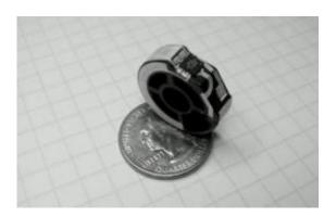
The Smart Connector, a new sensor device, is installed in the connecting units of coaxial cables to provide real-time information about primary failure modes in radio-frequency cables. Researchers in RIT's Kate Gleason College of Engineering and PPC, a Syracuse-based telecommunications connector equipment company, developed the device. Credit: Provided by Robert Bowman
