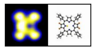
Physicists at the Technische Universitaet Muenchen have created a nano switch based on a single porphyrin ring. If one of two protons from the inside of the ring is removed, the remaining proton can take on any one of four positions, initiated by a single tunnel electron from the tip of a scanning tunneling microscope. Credit: Knud Seufert / Technische Universitaet Muenchen
