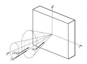
Volume holographic design of the fth of eight independent recordings used to generate the QT unitary transformation, U^QT, in PTR glass. For more information, please see the arxiv article.
