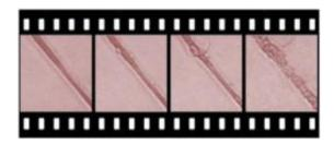
A series of transmission X-ray microscopy images obtained at different times in the course of the galvanic replacement reaction between a silver nanowire and an aqueous solution of HAuCl4, showing the morphological transformation of the solid nanowire into a hollow nanotube. Experiments were performed at the APS 32-ID-C beamline.
