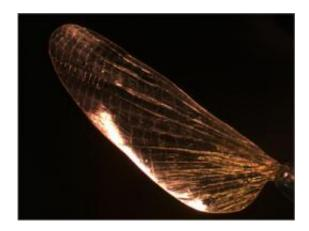
Shrilk is similar in strength and toughness to an aluminum alloy, but it is only half the weight. Shown here is a replica of a grasshopper wing, which was made with the new material.
