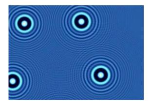
This hologram (false color added) displays the three-dimensional location of the polystyrene particles in a two-dimensional image. Credit: Ryan McGorty
