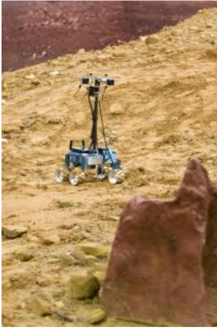
Robotic rover "indie" being tested on the simulated martian landscape
