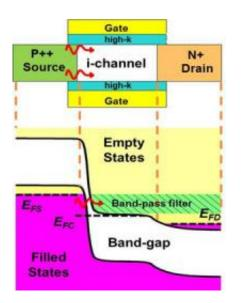
Schematic of the HTFET showing staggered band alignment. Credit: Penn State
