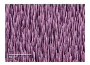
Colorized micrograph of multi-walled carbon nanotubes, each 40 micrometers long, which absorb more than 99.9 percent of the light inside NIST's prototype fiber-coupled radiometer. Credit: Huang/NanoLab, colorized by Talbott/NIST
