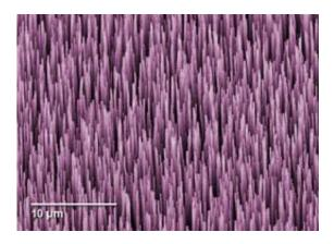
Colorized micrograph of multi-walled carbon nanotubes, each 40 micrometers long, which absorb more than 99.9 percent of the light inside NIST's prototype fiber-coupled radiometer. Credit: Huang/NanoLab, colorized by Talbott/NIST
