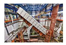
Engineers at Fermilab designed and tested a hydraulic system that will move and rotate 200-ton blocks of detector components for the assembly of the NOvA neutrino detector.
