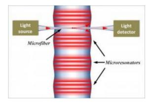
This figure is an illustration of SNAP microresonators formed by nanoscale variation of the optical fiber diameter. Credit: Courtesy OFS Laboratories.
