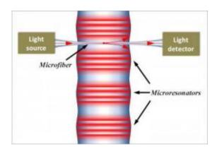
This figure is an illustration of SNAP microresonators formed by nanoscale variation of the optical fiber diameter. Credit: Courtesy OFS Laboratories.
