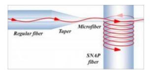
This figure shows the propagation of light in a SNAP fiber coupled to a tapered regular optical fiber. Credit: Courtesy OFS Laboratories
