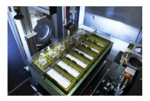
Adsorption trough assembly of the FIGARO neutron reflectometer at the ILL on which these air/liquid interface measurements were carried out. Credit: ILL/Alexis Chézičre
