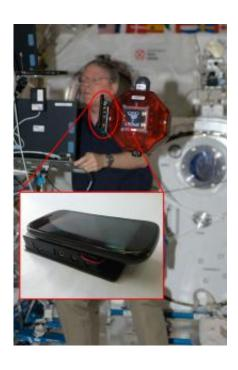
International Space Station researcher Mike Fossum, commander of Expedition 29, puts one of the Smart SPHERES through its paces. When viewing the large image, the inset image shows the Samsung Nexus S<sup>TM</sup> handset that helps turn the SPHERES into mobile data acquisition assistants for space explorers. Credit: NASA
