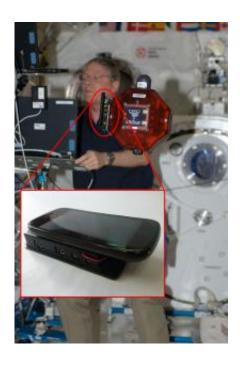
International Space Station researcher Mike Fossum, commander of Expedition 29, puts one of the Smart SPHERES through its paces. When viewing the large image, the inset image shows the Samsung Nexus S<sup>TM</sup> handset that helps turn the SPHERES into mobile data acquisition assistants for space explorers. Credit: NASA
