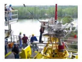
Stennis Space Center engineers and technicians install the J-2X powerpack into the A-1 test stand in preparation for testing Dec. 5. Credit: NASA/SSC
