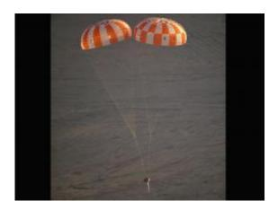
A test article that mimics the Orion spacecraft is seen under parachutes Tuesday as NASA engineers conducted a drop test above Yuma, Ariz. The Orion team was examining how the spacecraft would land under only two parachutes, instead of the normal three. Credit: NASA/James Blair
