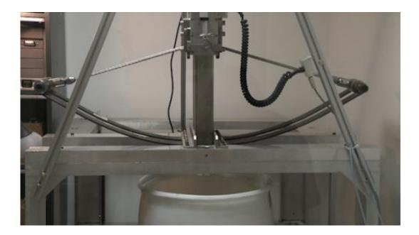
This is a photo of the ballista testbed preparing to fire a prototype harpoon into a bucket of material that simulates a comet. Credit: NASA/Rob Andreoli
