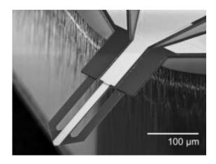
This is an electrothermal cantilever from the University of Illinois, having nanometer-scale electrode tip integrated onto a microheater. Credit: University of Illinois at Urbana-Champaign
