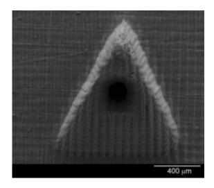
This is a scanning electron micrograph of a hollow microneedle, which was prepared out of an acrylate-based polymer. In this study, hollow microneedles were integrated with sensors for detection of glucose, lactate, and pH levels in a selective and simultaneous manner. Credit: Roger Narayan, North Carolina State University
