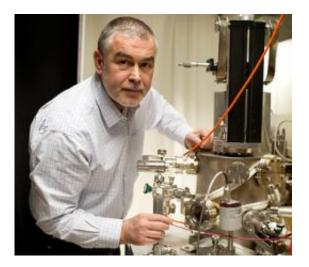
Dinko Chakarov with a laser-based vacuum system used to study the interaction between light and nanoparticles. Photo: Peter Widing / Chalmers
