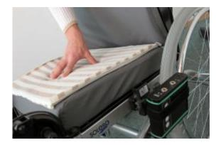
A sensor mat integrated in a wheelchair set helps prevent pressure ulcers. Credit: Fraunhofer IFF
