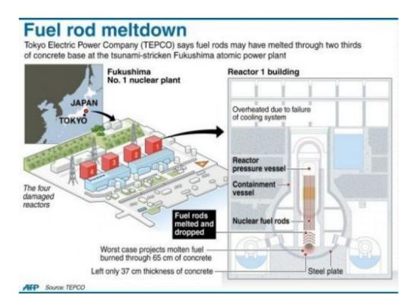
Graphic showing how molten fuel rods may have burned two thirds of the way through a concrete containment base, according to new information released by Tokyo Electric Power company.
