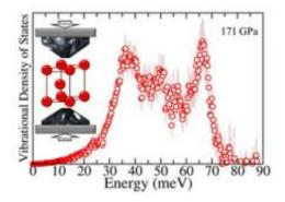
The vibrational spectrum of iron, the most abundant element in Earth's core, at 171 gigapascals. By squeezing iron between two diamond anvils (inset), Caltech researchers reproduced the pressures found in Earth's core. [Credit: Caitlin A. Murphy/Caltech]
