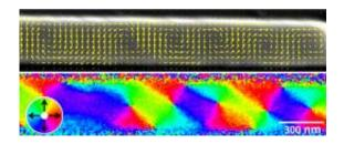
(PhysOrg.com) -- An international collaboration led by the NIST Center for Nanoscale Science and Technology has used scanning electron microscopy with polarization analysis (SEMPA) to acquire images of the magnetic structure inside patterned nickel-palladium (NiPd) thin film nanostructures, revealing peculiar magnetization textures that can affect the behavior of these ferromagnetic alloys in experimental applications.
