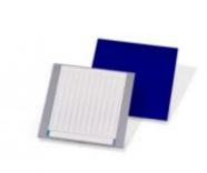
Caption: Interdigitated back-contact silicon solar cells above 23% efficiency
